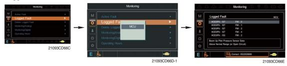
$\cdot\,$  The logged faults of the MCU can be checked by this menu.
